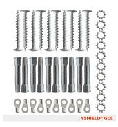
**Grounding set for the use with our magnetic shielding film MCL61.** The MCL61 surface is electrically insulated. Whilst screwing down the cable lug, the chopper disks will perforate the polyester film and arrange electrical contact thereby.
