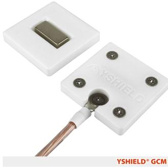
Grounding connection with two plates that hold together with the help of strong magnets. For all electrically conductive fabrics, fleeces, meshes. **The two connecting plates hold together magnetically - the material that is supposed to be grounded does not have to be perforated.**
